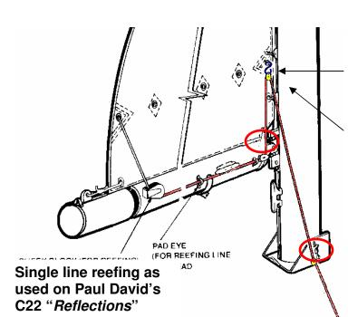
S hook in reef cringle – Reefing line runs through small block at bottom part of S hook – Nothing is fixed to anything at this area
